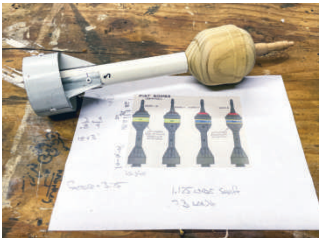
With the top of the round complete, it was time to build the fins. You can roughly cut the sheet metal bits with tin snips.
