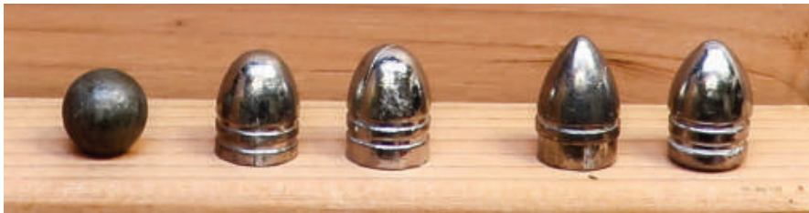
Bullets (above) for the Model 1860 Army .44 include 200- and 220-grain round-nosed Lee bullets, and Eras Gone Johnston & Dow and Kerr bullets. Colt Black Powder Arms 2nd Generation McCulloch 1860 and stainless steel 1860 (below) with Johnston & Dow cast bullets.
