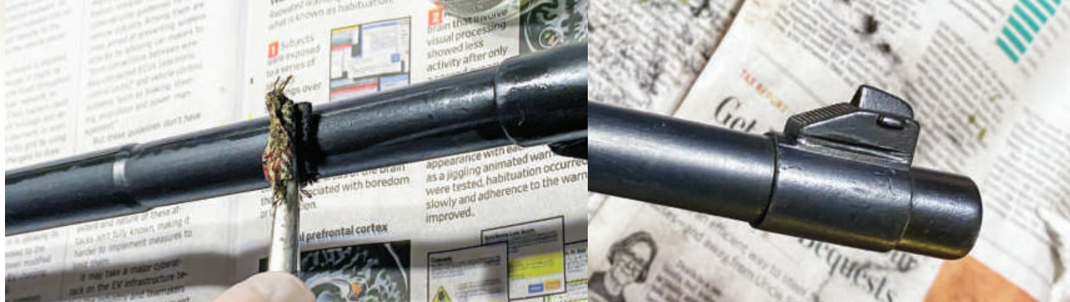
Apply the bluing solution (left) so it just moistens the surface of the metal without flowing or running. Use long strokes with minimal overlap and avoid rubbing excessively in any one spot. The side of this barrel (right) was polished to bare metal to remove an import mark, yet it took the blue as evenly as the patinaed metal.
