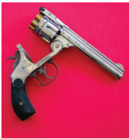
All Smith & Wesson models, whether double-action or single-action, featured a barrel/cylinder that allowed simultaneous ejection of fired cartridges.
