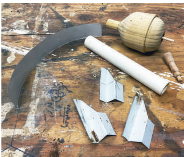
The warhead for Will's PIAT round began life as a wooden stair baluster (above) from Home Depot. The finished round (below) ready for painting looks undeniably crude.
