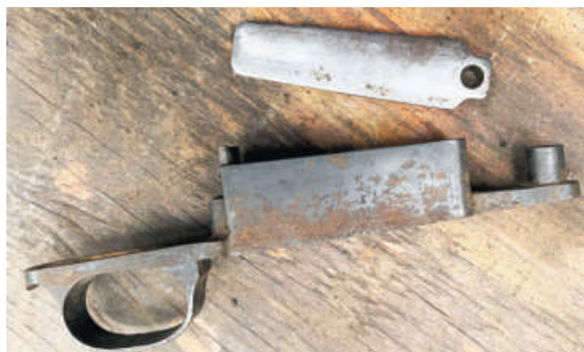
The trigger guard, like the barreled receiver, had some deep pitting. All of the active rust and compacted dirt and grease were removed from the metal before rust bluing. The same parts after clean-up on the wire wheel. Frank used small brushes and coarse steel wool to get inside the trigger guard and magazine box.
