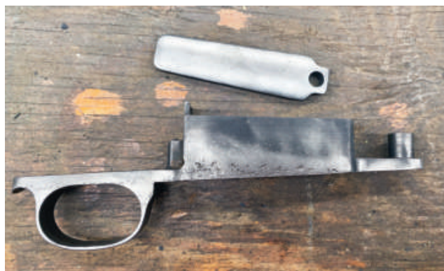
The trigger guard, like the barreled receiver, had some deep pitting. All of the active rust and compacted dirt and grease were removed from the metal before rust bluing. The same parts after clean-up on the wire wheel. Frank used small brushes and coarse steel wool to get inside the trigger guard and magazine box.
