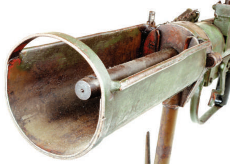
The PIAT was actually a spigot mortar. This spring-driven rod has a firing pin on the end that shoves up into the projectile.
