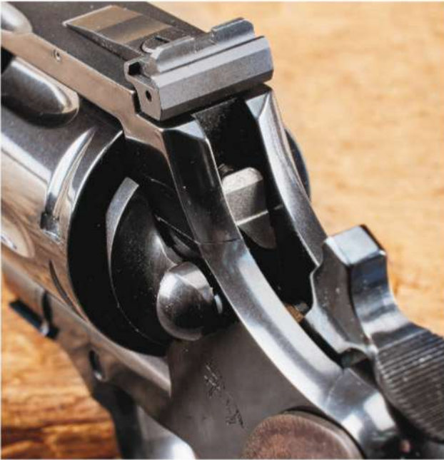
The Python utilizes a transfer-bar firing mechanism and a frame-mounted firing pin. Note the revolver's grooved hammerspur.
