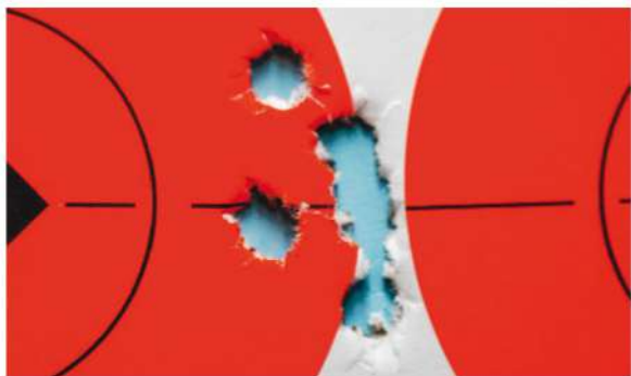
The Stevens Model 334 acquitted itself well on the shooting range, averaging 1.29-inch, five-shot groups at 100 yards with a total of 17 different .243 Win. loads. Steve says it's ready to hunt.
