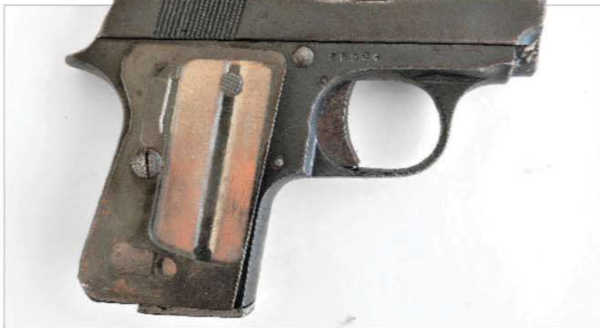
A The tiny Astra Cub was a six-shot .22 Short with rudimentary sights. At some point in its life a previous owner swapped the hard plastic grips for clear Lexan-type grips.
