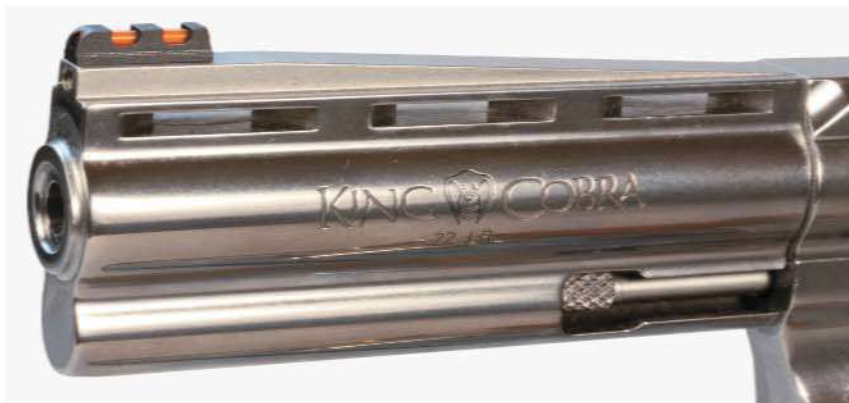
A The barrel has a full-length underlug for great balance. Unlike other guns in the line, the .22 has a ventilated rib. The top of the rib and frontstrap are matte-finished to eliminate glare.
