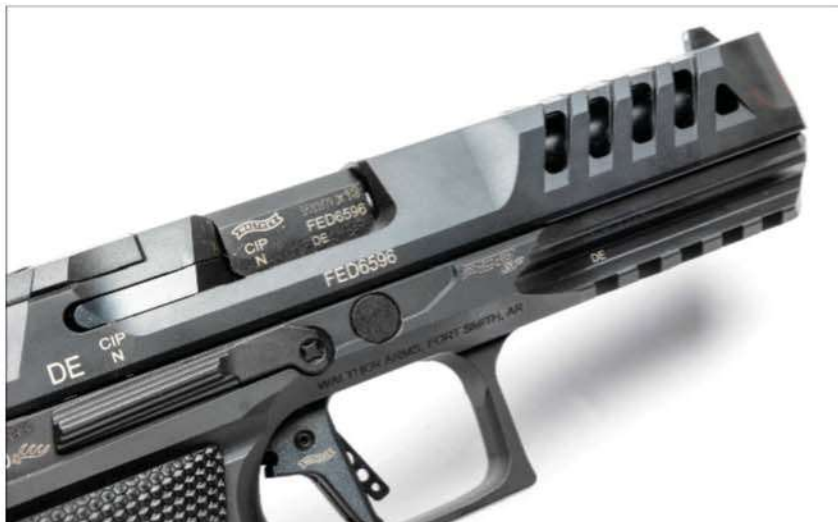
▲ Aggressive slide cuts reduce reciprocating weight and provide a positive grip for manipulating the slide, while on the steel gun the heavier accessory rail adds weight out front to help combat muzzle rise.
