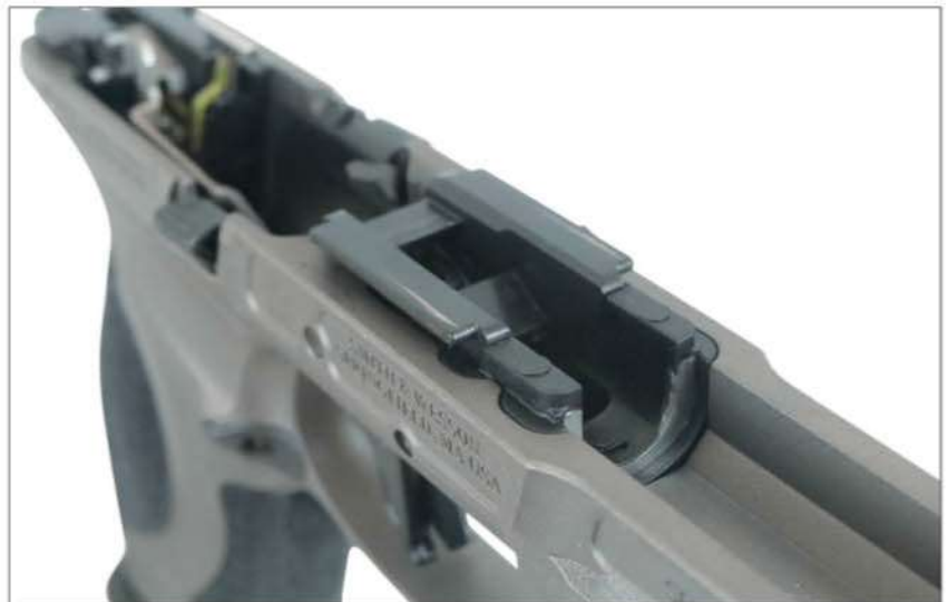
A The precision-machined, hand-fitted accuracy rail provides a consistent barrel/slide lockup, a big reason these guns shoot so well.
