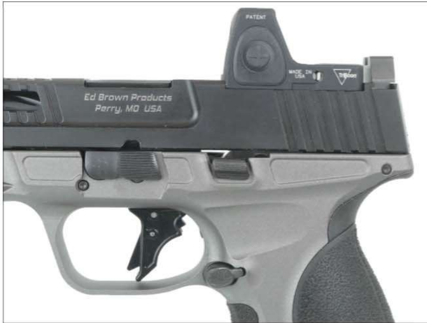
▲ The control layout on the Ed Brown Fueled series is standard S&W M&P9. There’s an ambidextrous slide stop, an oval magazine release and a rotating takedown lever.
